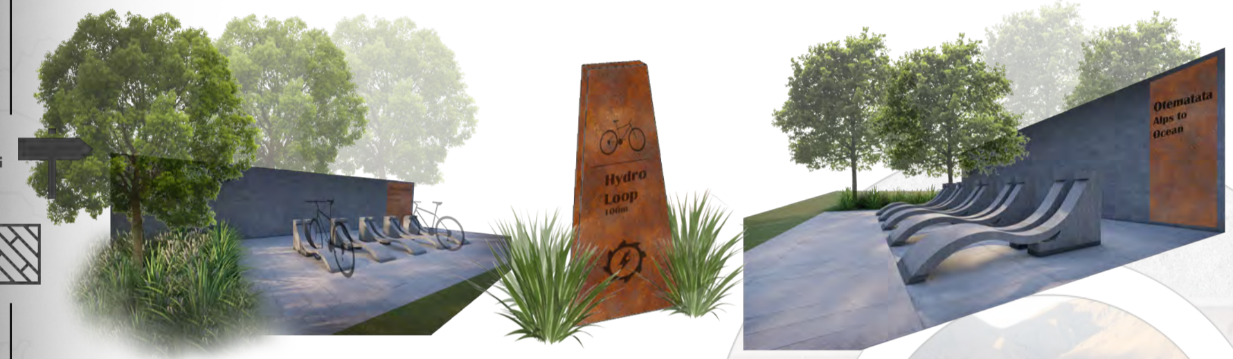
Bicycle stands and corresponding signage have been inspired by the Benmore and Aviemore hydro dams. The shapes and materials are set to replicate those prominent in hydro structures to create unique yet functional features. The use of both poured concrete and corten steel adds to an industrial aesthetic that contrasts surrounding natural hardwoods and stone.
